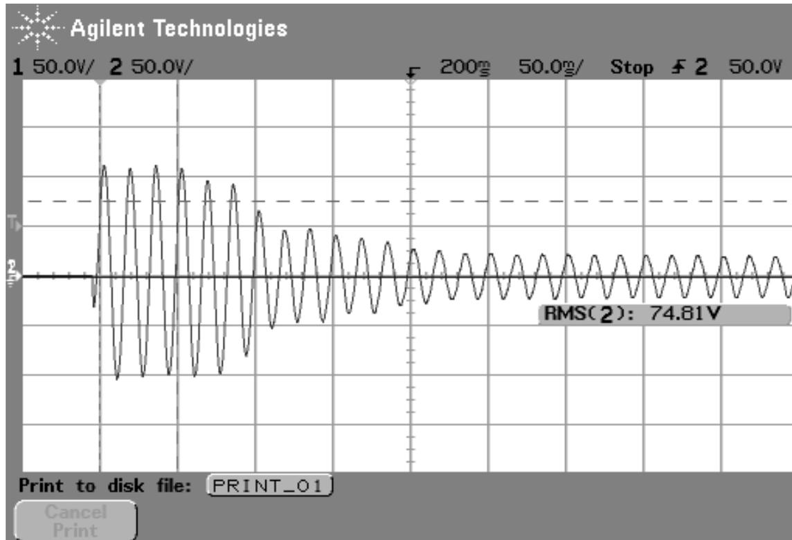
**Figure 5:** Starting current of air conditioner.
