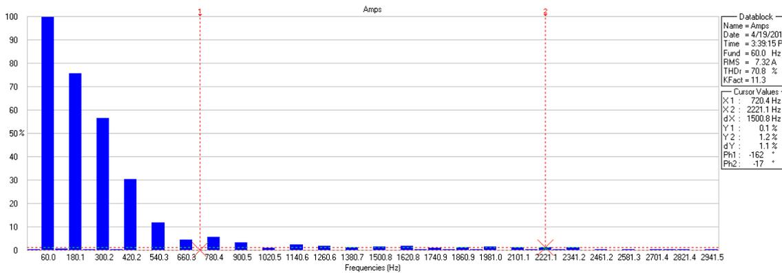
Figure 3: Harmonic distortion from switch-mode power supply.
