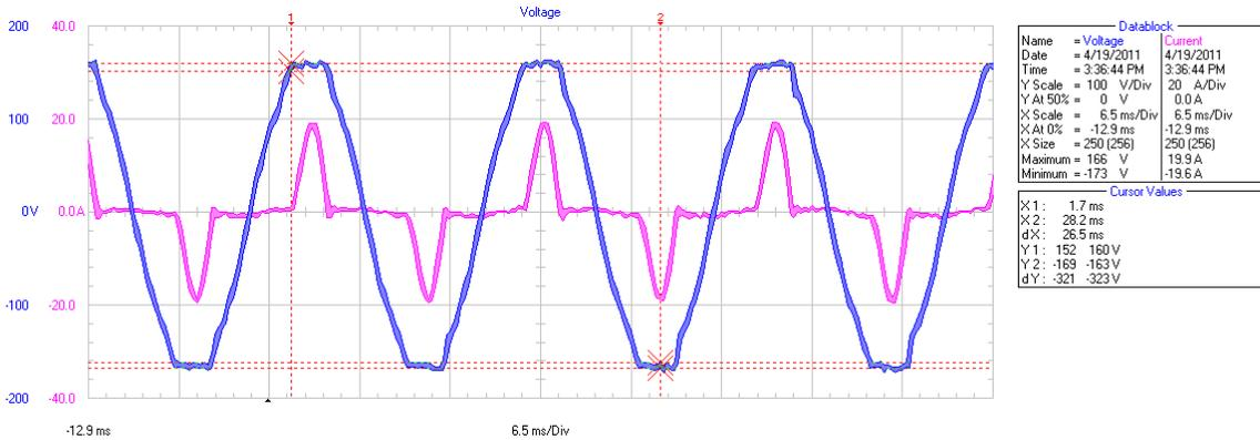
Figure 2: Voltage and current waveforms from switch-mode power supply.
