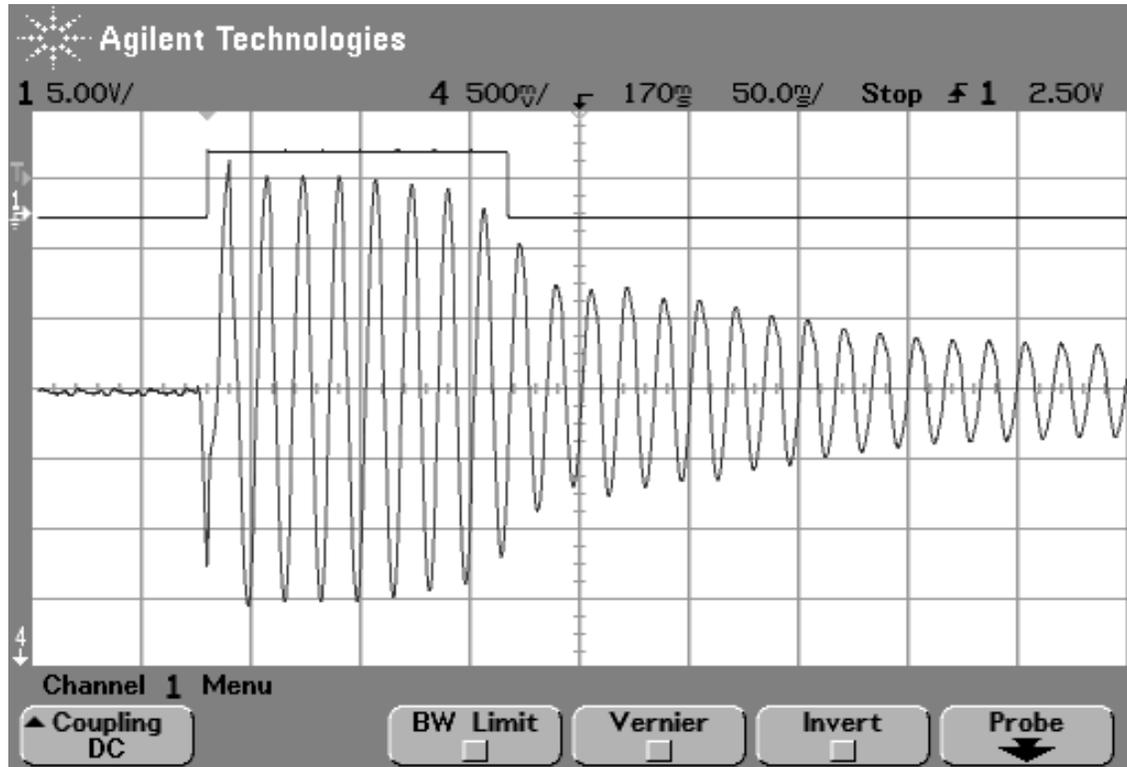
Figure 6: Air conditioner starting current supplied by Inverter 1.
