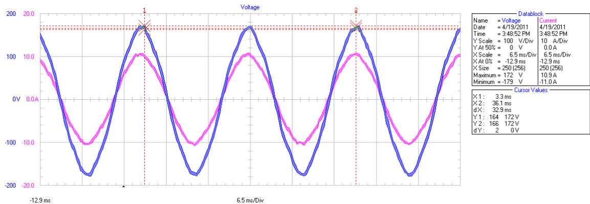
**Figure 4:** Voltage and current waveforms from resistive load.
