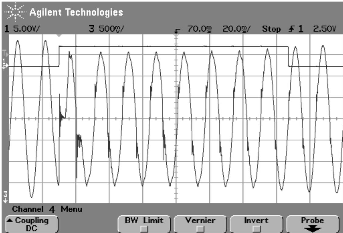
Figure 7: Air conditioner voltage supplied by Inverter 1.
