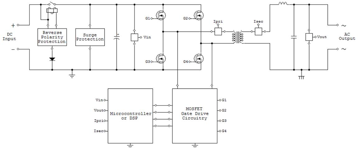
**Figure 9:** Typical inverter block diagram.
