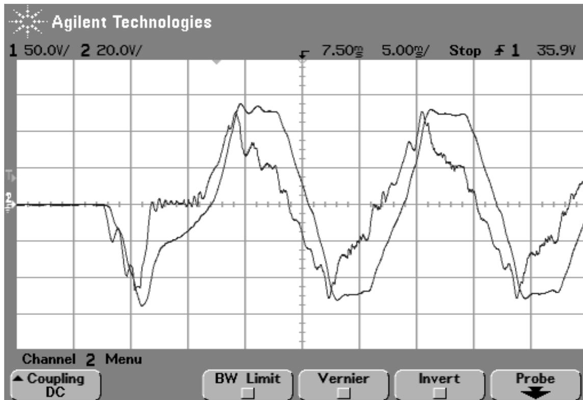
**Figure 8:** Air conditioner current and voltage waveforms from Inverter 2.
